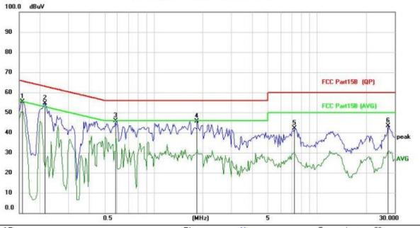
Site LAB Phase: Ν Temperature: 26 Limit: FCC Part15B (QP) Humidity: 60 % Power:
